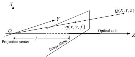
Figure 4. Linear camera models
