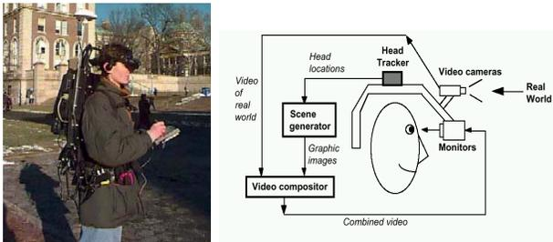
Figure 6 the UAV operator with augmented reality equipment and its structure
