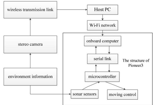
Figure 12. The Overall Structure of Obstacle Avoidance Test System
