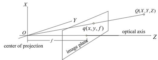
Figure 1. The Model of Pinhole Camera
