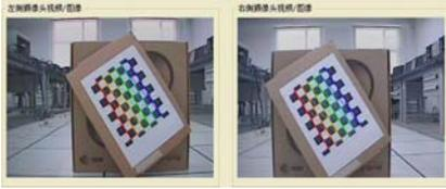
Figure 2. Stereo Calibration Pictures
