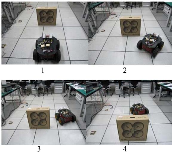
Figure 14. Obstacle Avoidance Processing
